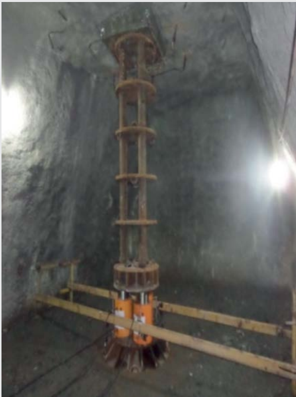
FIGURE 2 - Stress-path test in an adit at Cihaxia site
